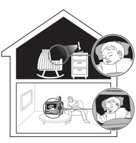
The baby unit has infrared LEDs that allow you to see your baby clearly at night or in a dark room. When the baby unit detects low light levels, the infrared LEDs are switched on automatically. The images from the baby unit are in black and white, and appears on the parent unit screen.
