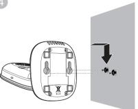
Align the wall mount holes on the baby unit with the screws on the wall. Slide the baby unit down until it locks
