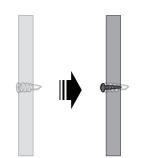
tighten the screws until only 6.5 mm of the screws are exposed.
