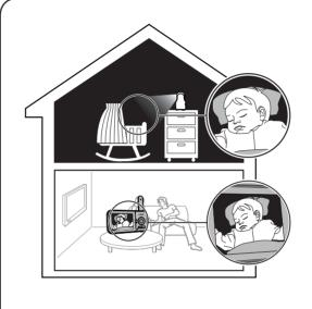
The baby unit has infrared LEDs that allow you to see your baby clearly at night or in a dark room. When the baby unit being viewed detects low light levels, the infrared LEDs are switched on automatically. The images from the baby unit are in black and white, and 🥹 appears on the screen.
