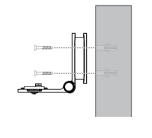
. Insert the screws into the holes and tighten the screws until only 6.5 mm of the screws are exposed.
