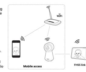
Internet connectivity to your HD video monitor system. It serves as a communication channel between your baby unit and mobile device, allowing you to monitor and/or control your baby unit wherever you are. For more details, see **Download app for mobile access** section in this quick start guide.
